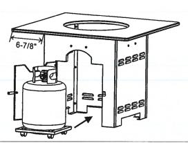
Center the granite table top on the top of the steel base, the granite should hang over the edge of the steel base by approximately 6-7/8"on all 4 sides.
