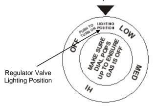
If the burner does not light before 7 seconds of clicking, turn the regulator OR valve to the OFF position and wait 5 minutes for the gas to clear before trying again.
