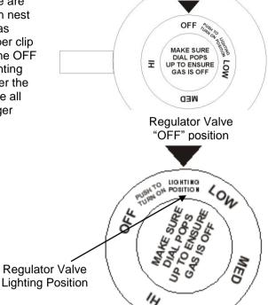
If the burner does not light before 7 seconds of clicking, turn the regulator to the OFF position and wait 5 minutes for the gas to clear before trying again.
