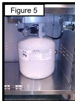
9. Open tank valve **SLOWLY** (counterclockwise) until fully open. Use a soapy water solution to check all connections for leaks before lighting grill. If a leak is found **DO NOT** use the grill. Turn gas off and call a professional gas fitter to repair the leak.
