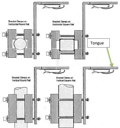
Figure 3: Rail Mount (Horizontal and Vertical Mount)
